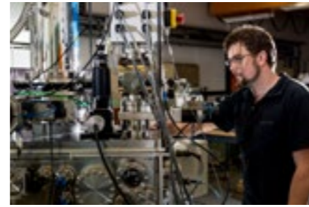
▲ The Sensitive High Resolution Ion Microprobe (SHRIMP) for analysing geological materials was designed and developed at ANU.
